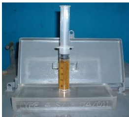
Figure 2. Live Tank Oil Sampling (swop with LTOS sampling image from the sales brochure)
