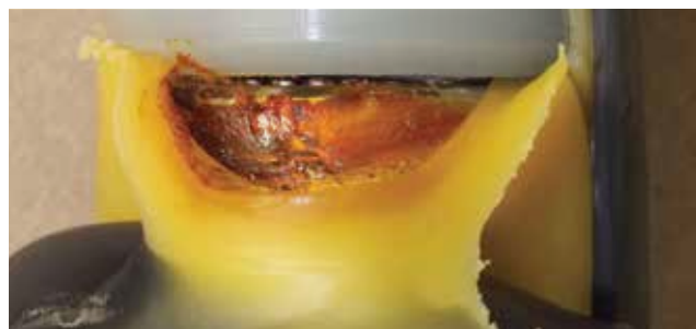
One of the three HV cables at the Grangemouth site where routine testing revealed critical PD activity.
