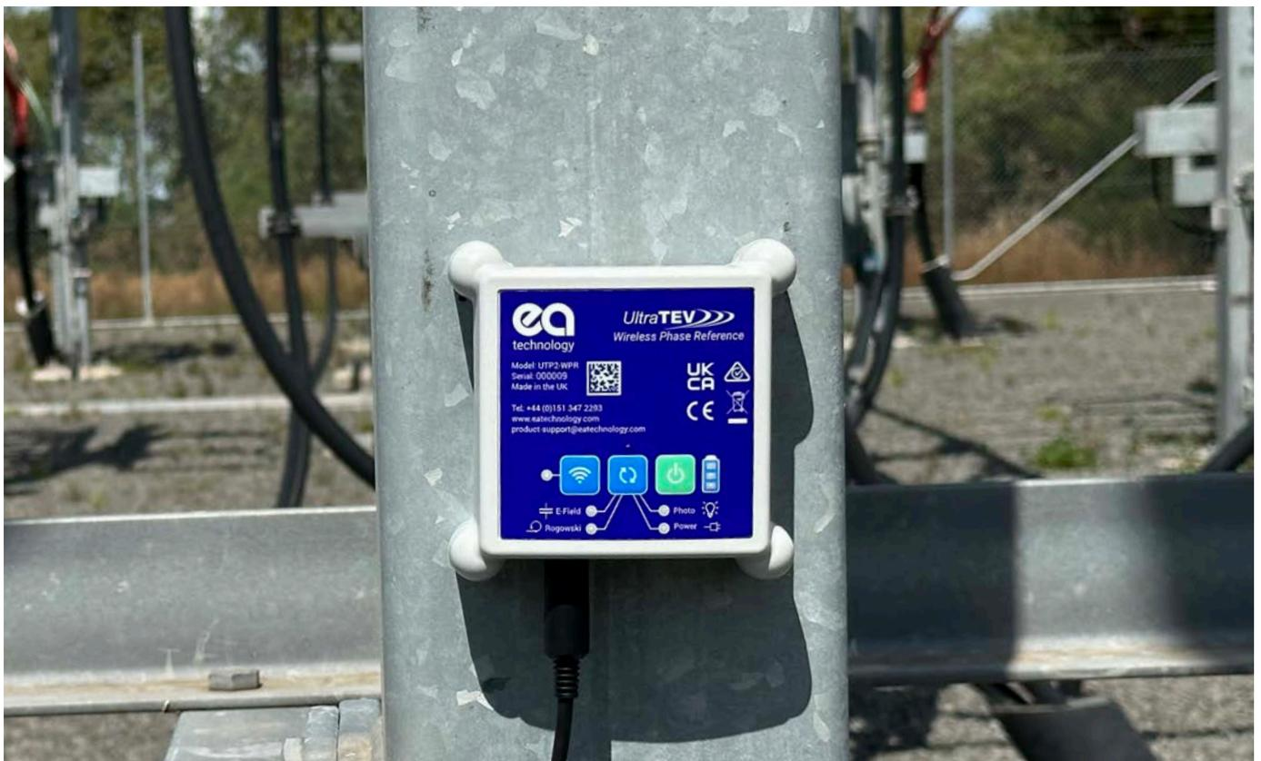
Wireless Phase Reference being used in situation.
