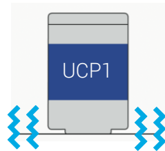
Vibration (including transformers) of asset enclosure where the UCP1 is attached
