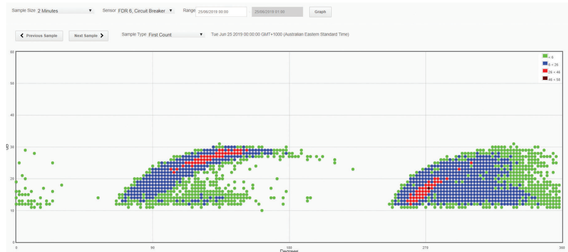
Figure 5: Phase Resolved Plot Showing Significant PD
